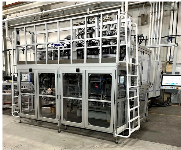
Uniloy’s 24-cavity, in-line reciprocating screw blow molding system — the largest of its kind in the industry.
